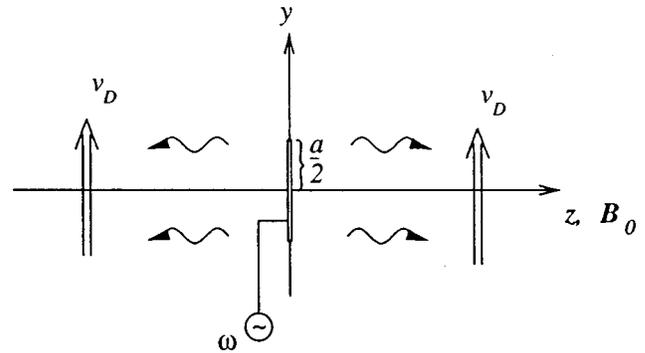
FIG. 2. Schematic of excitation model. A transparent strip exciter of width  $a$  (on the order of the electron skin-depth) is modulated by a generator at frequency  $\omega$  in a plasma with a bulk flow velocity  $v_D$  along the positive  $z$  direction. The confining magnetic field  $B_0$  is perpendicular to the exciter.
