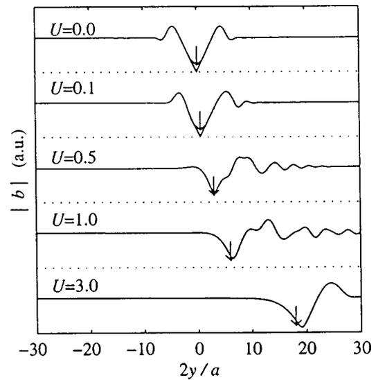
FIG. 4. Effect of increasing scaled drift-velocity on transverse spatial dependence of magnitude of scaled magnetic field at fixed scaled axial position  $\xi=6.0$ ;  $p=1.0$ . Arrow indicates location of center of current channel predicted by ideal MHD. Dotted lines are zero baseline for curves immediately above.
