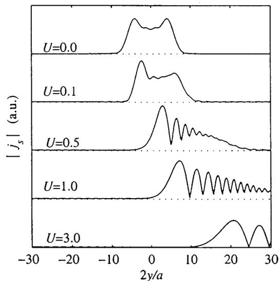
FIG. 5. Transverse spatial dependence of the magnitude of the scaled axial current density for different scaled flow speeds  $U$  at a fixed axial position  $\xi = 6.0$ ;  $p = 1.0$ .
