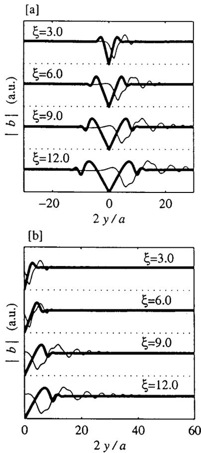
FIG. 3. Transverse spatial dependence of magnitude of scaled magnetic field for different axial positions. Heavier curves are in the absence of flow, and lighter curves when  $U=0.5$ . (b) is the same as (a) but over an expanded transverse distance.  $p=1.0$ . Dotted line is zero baseline for curves immediately above.
