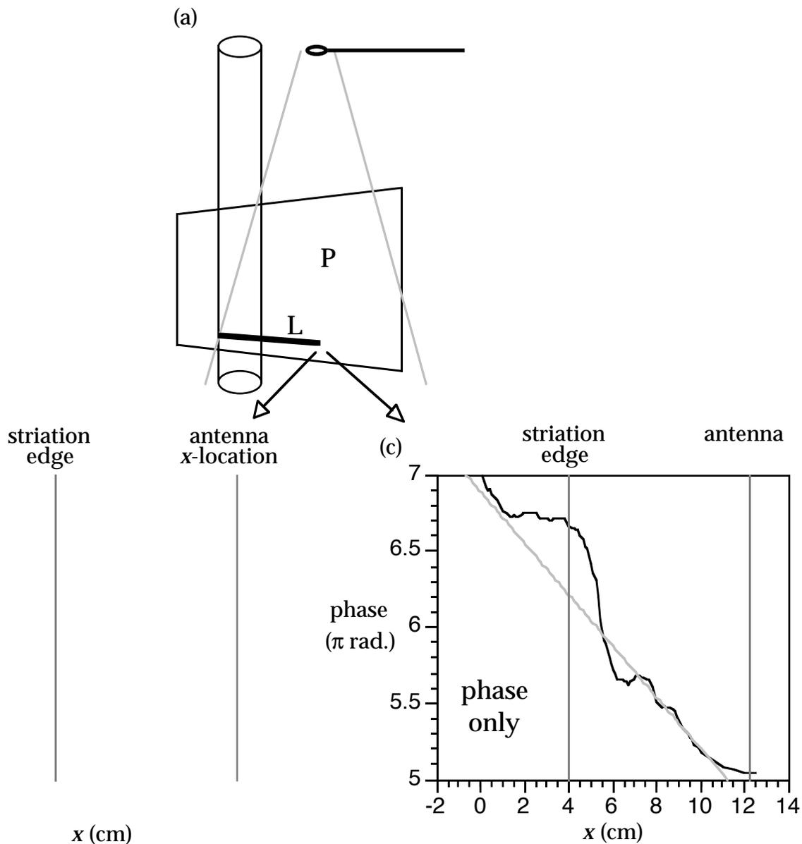
**Figure 5.** 1-D  $B_z$  data separated into amplitude and phase components. A schematic diagram (a) shows the spatial relationship between the antenna, striation, data plane (P) and a linear subset of the data (L) in the interaction region. The amplitude-only data,  $|B_z|$ , are shown in (b) and the phase-only data in (c) which also contains a straight line fit to the data calculated for the region  $7 < x < 10$  cm. The slope of this line yields the incident whistler
