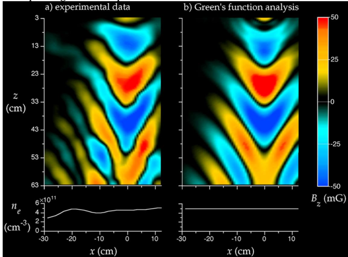
**Plate 3.** Comparison of Green's function predicted antenna radiation pattern with experimental data taken in a nearly uniform plasma. The pattern is calculated for the following experimental parameters: a magnetic field of 540 G, a frequency of 80 MHz, and a density of  $5 \times 10^{11} \text{ cm}^{-3}$ . The antenna is located at the origin, but 5 cm above the data planes shown here. The view is
