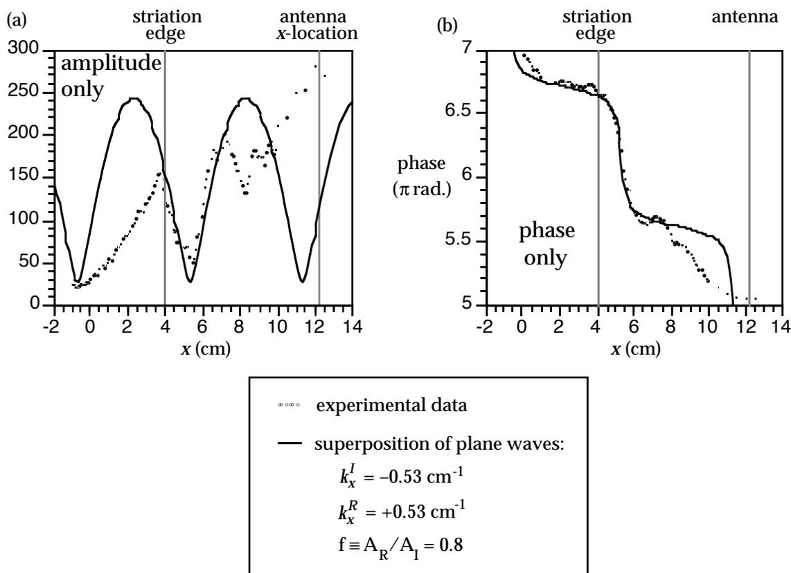
**Figure 6.** Comparison of experimental data with the superposition of two oppositely directed plane waves. The data are decomposed into amplitude (a) and phase (b) components for the same linear subset as in Fig. 5. The plane waves are meant to represent the incident and reflected whistler waves. Wave numbers and relative amplitudes of the two plane waves are adjusted to give the best fit in the region  $4 < x < 8$  cm. The result is wave numbers of
