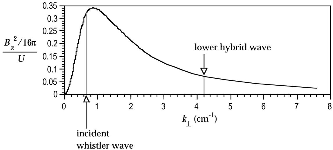
**Figure 7.** Fraction of wave energy density contained in the wave  $B_z$  component as a function of  $k_\perp$ . The fraction of the wave energy density peaks at a  $k_\perp$  value near that of the incident whistler wave. At typical lower hybrid wave  $k_\perp$  values, the fraction is about 5 times lower.
