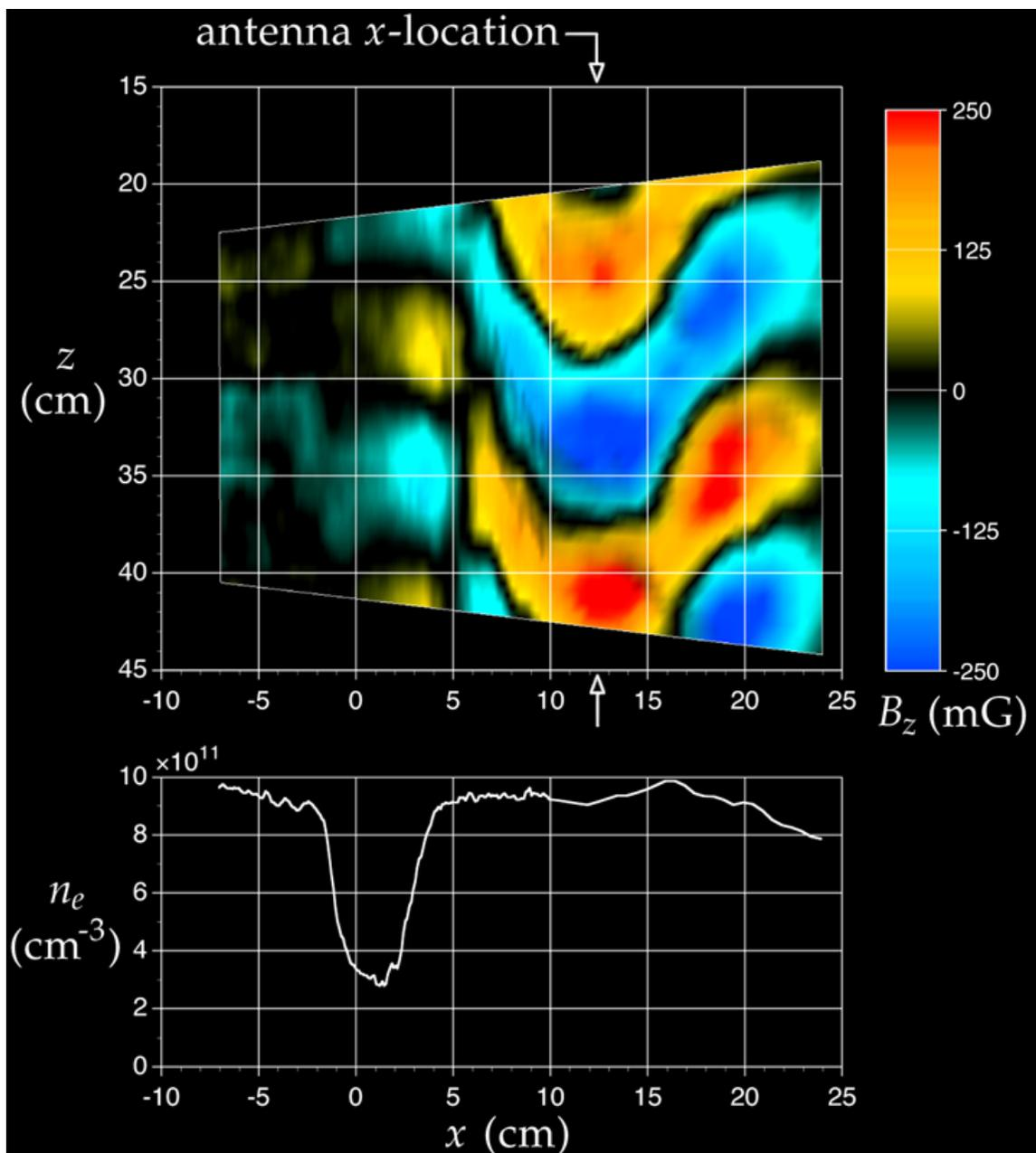
**Plate 4.** Measured  $B_z$  wave field data in a 2-D  $(x, z)$  plane through the center of the density striation. The view is perpendicular to the background magnetic field. A radial profile of the plasma density is shown below for reference. The edge of the striation is at  $x = 3.8$  cm. The antenna  $x$ -location is indicated with arrows at  $x = 12.2$  cm.
