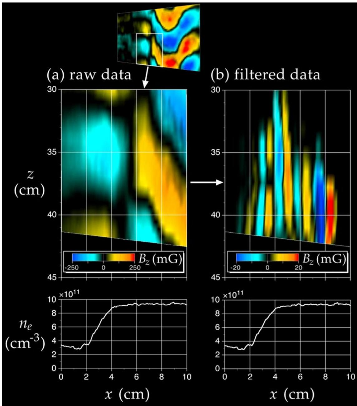
**Plate 5.** Detailed view of measured  $B_z$  wave field data in the interaction region. Data are shown raw in (a) and with long wavelengths filtered out in (b). The filtering process is described in detail in the text. As in Plate 4, the view is perpendicular to the background magnetic field and radial profiles of the plasma density are given below for reference. When the long wavelength,
