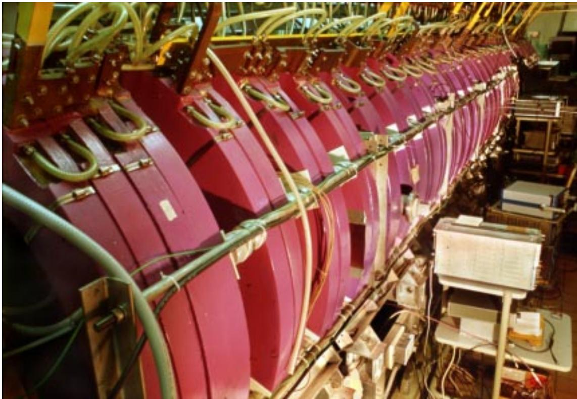
**Plate 1.** Photograph of the Large Plasma Device (LAPD) at UCLA. Visible in this photograph are the 68 magnet pairs which surround the 10 m long, 1 m diameter plasma chamber. Power and cooling water for the magnets are fed in from above. The cathode, which produces the DC discharge plasma, is located inside the far end of the machine. The plasma is accessible to probes through ports between the magnet pairs.
