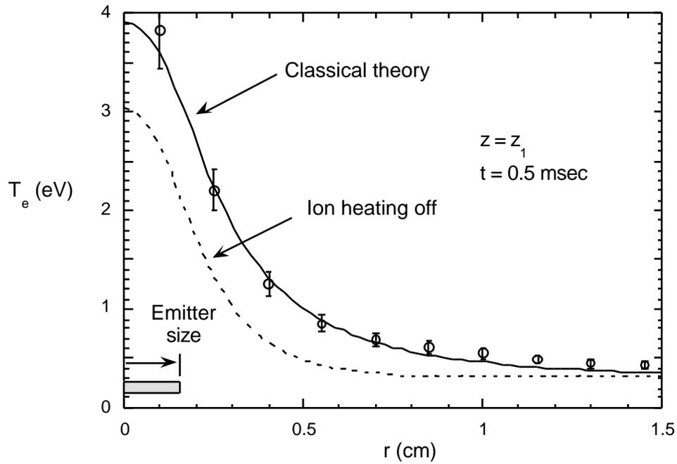
Fig. 3. Comparison of measured radial temperature profile (open circles) to the classical prediction (smooth continuous curve) at axial location  $z_1$ , 0.5 ms after beam turn on. The dashed curve is the predicted profile when the ion heating source in Eq. (2) is zero.
