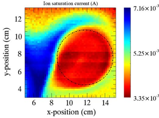
**Figure 10.** Time-averaged ion saturation current measured on Mach probe collecting surface facing toward the plasma source. The MDE and mesh anode biases are  $\Delta V_{\text{MDE}} = 420$  V and  $\Delta V_A = 40$  V, respectively, with  $B_0 = 1$  kG. Each square super-pixel represents a datum.
