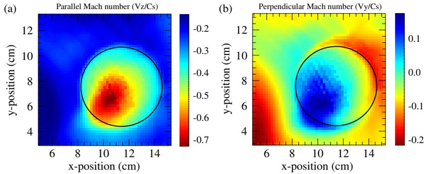
**Figure 9.** Parallel (a) and perpendicular (b) ion flow measured with a Mach probe. The dashed-dotted line represents the boundary of the mesh anode. The MDE and mesh anode biases are  $\Delta V_{\text{MDE}} = 420$  V and  $\Delta V_A = 40$  V, respectively, with  $B_0 = 1$  kG. Each square super-pixel represents a datum.
