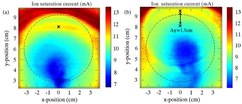
**Figure 12.** Ion saturation current measured on mach probe collecting surfaces facing toward the plasma source (a) at  $\Delta z = 2.88$  m and (b) at  $\Delta z = 1.92$  m ( $\Delta z$  is the axial distance from the mesh anode to the probe). The MDE and mesh-anode biases are  $\Delta V_{\text{MDE}} = 80$  V and  $\Delta V_A = 40$  V, respectively, with  $B_0 = 1$  kG. Each square super-pixel represents a datum.
