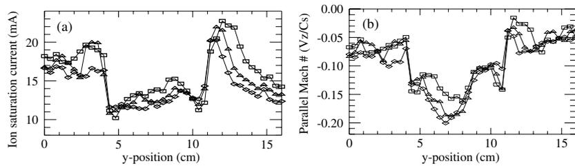
**Figure 6.** An off-axis (in  $y$ -direction) current channel (density depletion) (a) is created by applying a voltage drop between a copper mesh electrode and the plasma source anode ( $\Delta V = 40$  V (diamonds), 60 V (triangles) and 80 V (squares)). The parallel ion drift (b) was measured using a mach probe.
