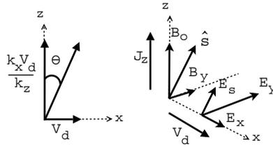
**Figure 1.** Cartesian geometry of the stationary Alfvén wave model with a depiction of the relevant field and initial flow vectors. For the case shown,  $k_x \gg k_y$  and  $J_z$  parallel to  $B_0$  (as opposed to antiparallel), the wavevector is angled slightly below and approximately parallel to the vector  $v_d$ . The angle in the leftmost coordinate system depicts the orientation of the effective phase velocity vector, as shown, and is approximately zero.
