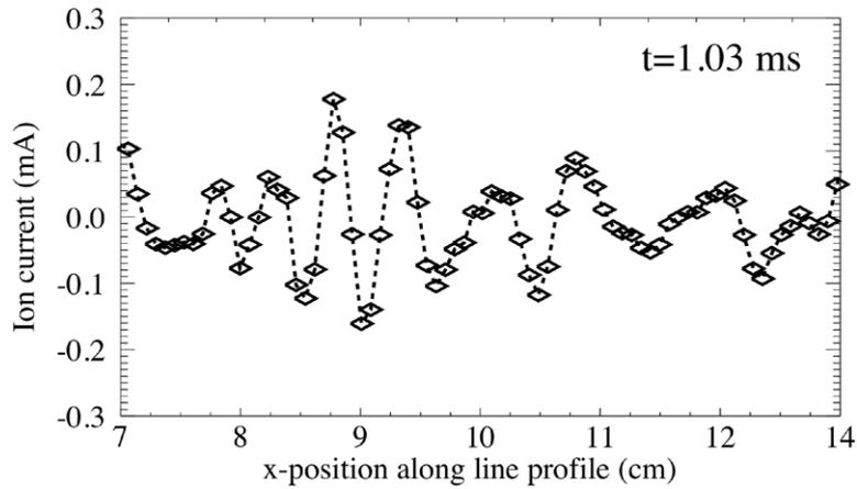
**Figure 4.** Linear interpolation of the measured values of ion saturation current lying along the dashed line in figure 3, plotted as a function of their  $x$ -coordinate.
