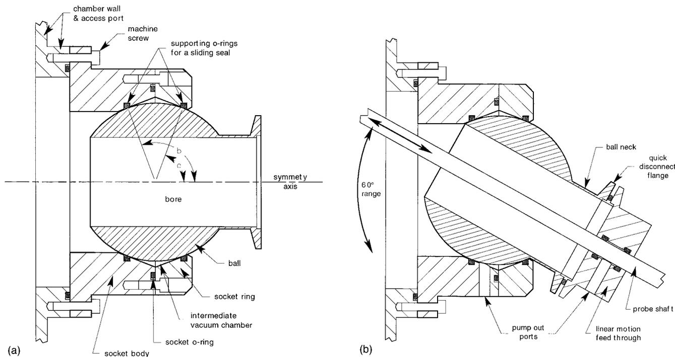
FIG. 1. Mechanical drawing of angular motion feedthrough. (a) The mechanism is in the axially aligned state showing the essential features of the design, i.e., the ball, the two component socket, the supporting O-rings for a sliding seal, and the differentially pumped intermediate vacuum chamber. (b) The mechanism is shown in an off-axis state. Additional design features are included: the linear motion vacuum feedthrough and the pump out ports for the differentially pumped chambers.
