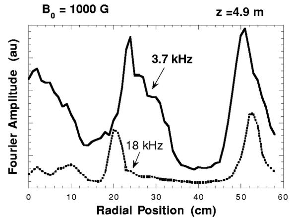
FIG. 14. The profiles of the spectral amplitude of low frequency noise are shown for two frequencies, 3.7 kHz (solid curve) and 18 kHz (dashed curve). The noise at 18 kHz corresponds to drift-Alfvén waves driven by steep gradients and is therefore spatially localized. The noise at 3.7 kHz corresponds to evanescent shear Alfvén waves driven by gentle gradients. These waves have a much broader spatial distribution.
