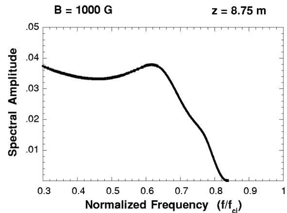
FIG. 16. Predicted spectral amplitude at axial location  $z=8.75$  m for  $B_0=1000$  G in the main plasma column. The model consists of partial wave reflections between cathode and anode where the average magnetic field is smaller than in the main column. To be compared to Fig. 9.
