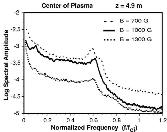
FIG. 5. Scaling of frequency spectra (log scale) at the center of the plasma with strength of the uniform confinement field  $B_0$  over the range of 700–1300 G. The frequency  $f$  is normalized to the ion cyclotron frequency  $f_{ci}$  to test for universality. The shape of the spectra does not change with  $B_0$ , but the absolute level of the fluctuations exhibits a favorable decrease with increasing  $B_0$ .  $z=4.9$  m and  $x=39$  cm.
