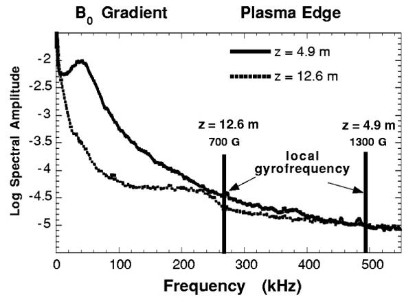
FIG. 11. Frequency spectra (log scale) at the plasma edge ( $x=56$  cm) in the presence of a linear axial gradient in the confinement magnetic field, as in Fig. 10.
