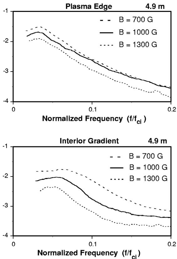
FIG. 7. Comparison of the spectra of magnetic field fluctuations at the plasma edge, in contact with metallic walls (top panel), to that generated within the interior gradient (bottom panel), surrounded by plasma.  $B_0$  is varied from 700 to 1300 G,  $z = 4.9$  m.
