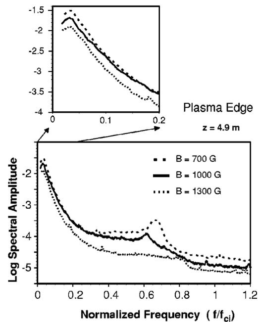
FIG. 6. Scaling of frequency spectra (log scale) at the plasma edge with strength of the uniform confinement field  $B_0$  over the range of 700–1300 G, as in Fig. 5. In this spatial region the shape of the spectrum for frequencies below  $0.25 f_{ci}$  is invariant and displays an exponential tail, but the details of the spectral shape vary at the higher frequencies. The decrease in fluctuation amplitude with increasing  $B_0$  is also found at the plasma edge.
