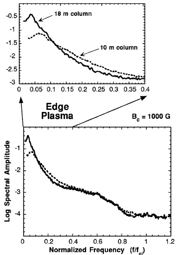
FIG. 8. Dependence of frequency spectra (log scale) at the plasma edge on the axial length of the plasma column. The solid curve is for 18 m column and the dotted curve is for 10 m. The spectra above  $0.2 f_{ci}$  is insensitive to column length. The top insert presents an expanded view of the lower frequency band. It shows a small shift toward lower frequencies for the longer column, as is expected for axially standing drift-Alfvén modes.  $z = 8.75$  m,  $x = 53$  cm, and  $B_0 = 1000$  G.
