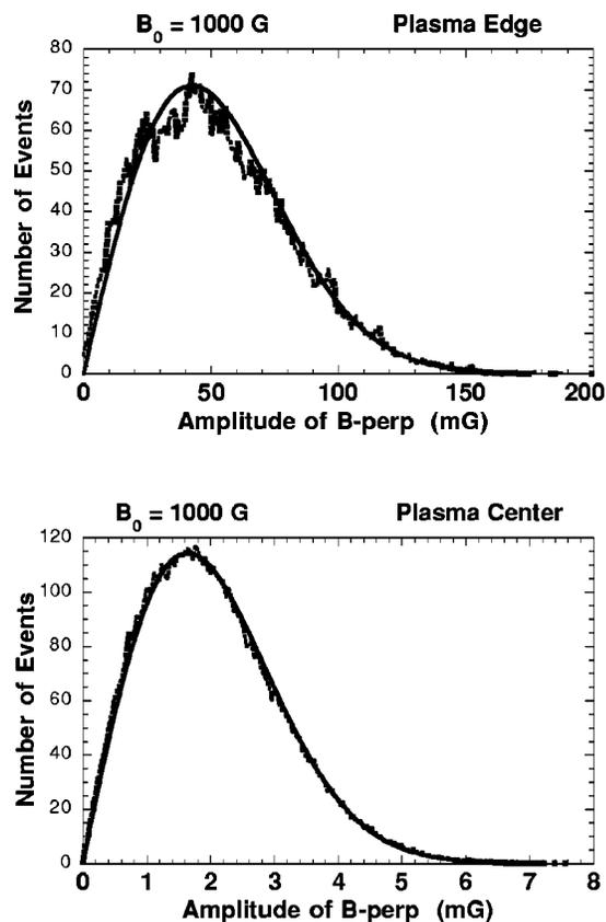
FIG. 15. Statistical properties of spontaneous magnetic field fluctuations observed under various conditions. Top: plasma edge at  $B_0 = 1000$  G, bottom: plasma center at  $B_0 = 1000$  G. The solid curve is a fitted Gaussian distribution and the dotted curve is data.
