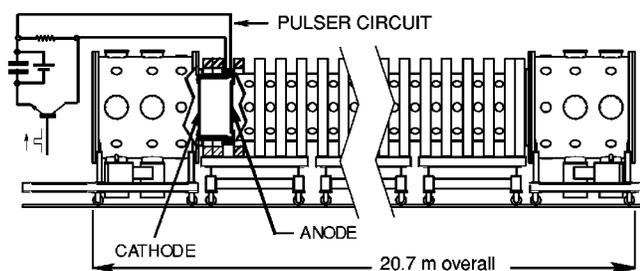
FIG. 1. A truncated schematic of the LAPD-U showing some of the vacuum chamber and axial field magnets, a cutaway of the source region, and the discharge pulser circuit.
