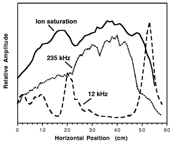
FIG. 3. Spatial dependence along the horizontal  $x$ -direction of the ion saturation current (top solid curve). In the regime of operation the ion saturation current essentially represents the plasma density. For comparison, the spatial behavior of the prominent spectral peaks at 12 kHz (dashed curve) and 235 kHz (dotted curve) identified later in Fig. 4 are also shown. The linear scales for each curve are adjusted to facilitate visualization.
