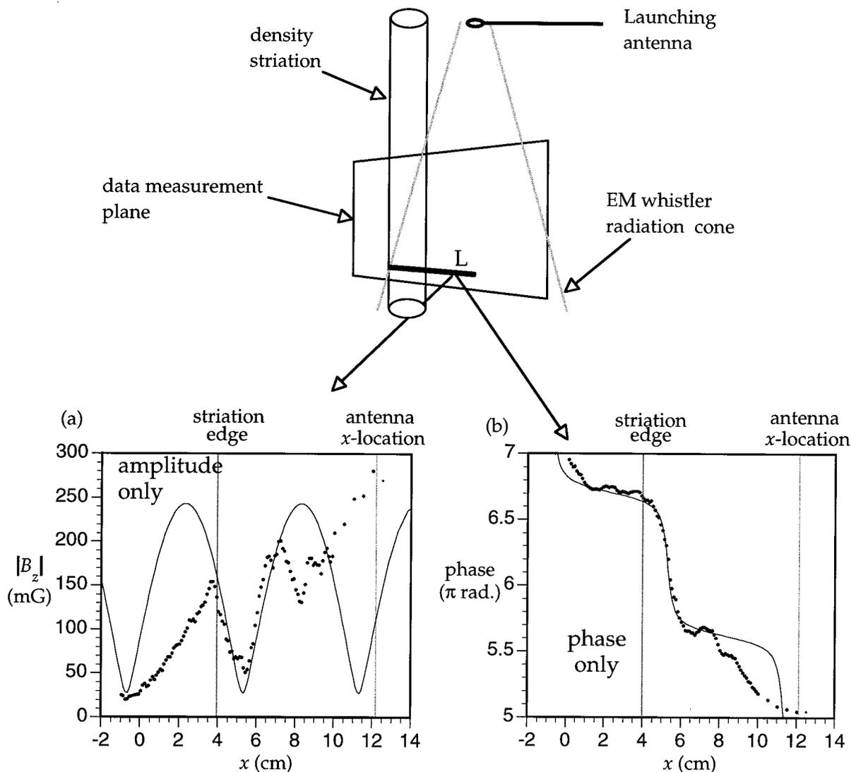
FIG. 8. A schematic of the geometry used in the whistler–striation interaction experiment showing the relative location of the measurement plane, striation, and launching antenna together with the (a) measured wave amplitude and (b) phase.
