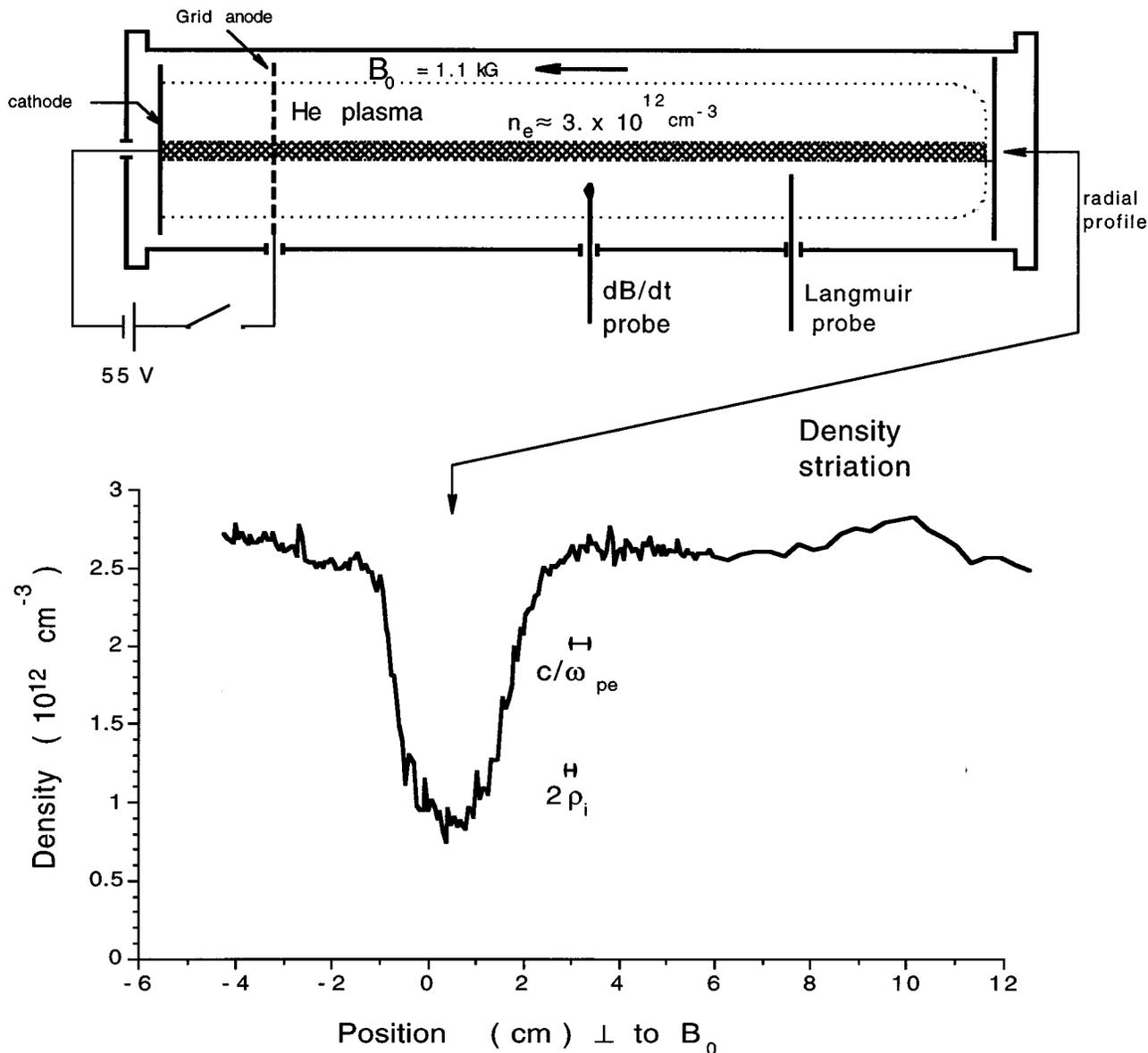
FIG. 1. A schematic of the geometry used in studying the spontaneous growth of magnetic fluctuations and a radial density profile through the center of the striation.
