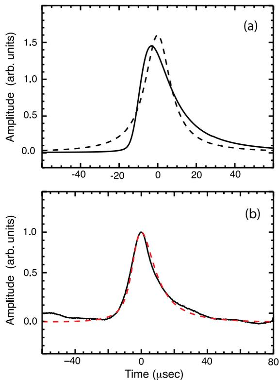
FIG. 3 (color online). (a) Skewed Lorentzian pulse (solid curve) with a pronounced “leading edge” ( $s = -0.8$ ) is compared to a symmetric pulse (dashed curve) with the same width,  $8 \mu\text{s}$ . (b) An experimentally observed pulse (solid line) is compared to a pulse generated from the inverse Fourier transform of  $\tilde{L}(\omega)$  (dashed curve).
