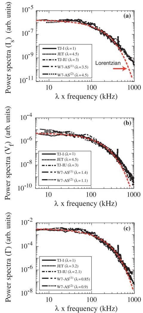
FIG. 5 (color). Power spectra of fluctuations in ion saturation current (a), floating potential (b), and turbulent flux (c) from the survey of Pedrosa *et al.* (black) (used with permission from [22]) is compared to the power spectrum of a single Lorentzian pulse with width,  $\tau = 1 \mu s$  (red dotted lines). The power spectra are clearly exponential for frequencies below 400 kHz, and the turbulent flux spectra is exponential over nearly the entire frequency range displayed.
