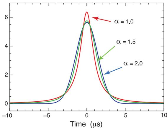
FIG. 1 (color). Examples of pulse shapes for three values of the parameter  $\alpha$  in Eq. (3). Gaussian is  $\alpha = 2.0$ , Lorentzian is  $\alpha = 1.0$ , and intermediate shape  $\alpha = 1.5$ . The “tails” of the pulses become more prominent as  $\alpha$  decreases from 2.0 to 1.0. All pulses have the same width,  $\tau = 1.0 \mu\text{s}$ .
