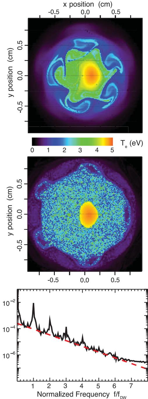
FIG. 4 (color). Results of a deterministic-chaos model. Top: Temperature contours in a filament just before the onset of chaotic behavior. Middle: Contours after the onset of chaos. Bottom: Power spectrum of temperature fluctuations corresponding to the middle panel.  $f_{DW}$  is the drift wave frequency.
