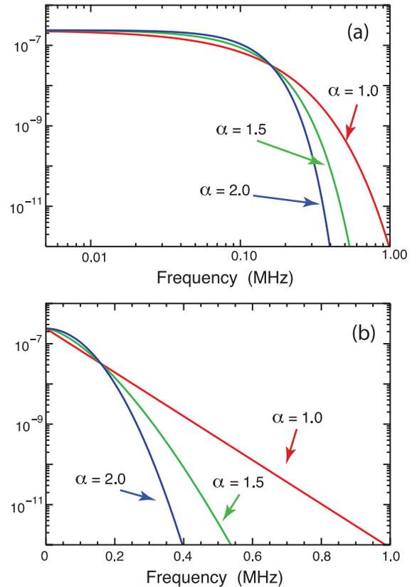
FIG. 2 (color). (a) Power spectra of the pulse shapes in Fig. 1 in a double-logarithmic format. (b) Same spectra in a log-linear format. The exponential spectrum is easily identified as a straight line in the log-linear format.
