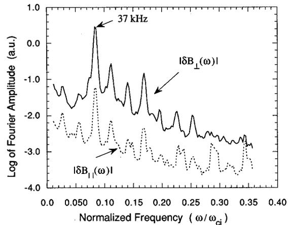
FIG. 11. Frequency spectrum of magnetic field fluctuations perpendicular to the background magnetic field compared to the spectrum of fluctuations parallel to the background field.
