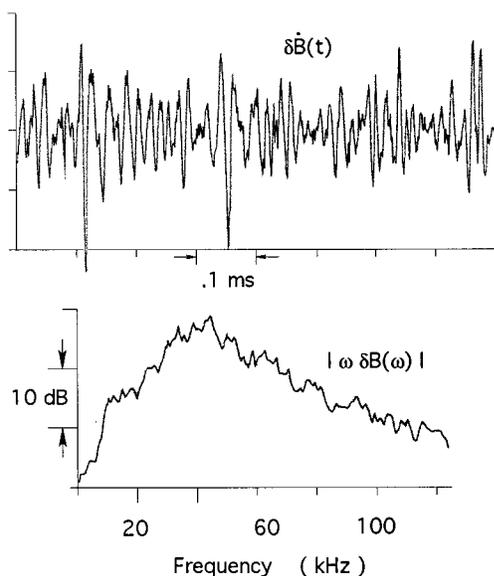
FIG. 14. Single-shot temporal behavior and frequency spectrum (ensemble average) of the time derivative of the magnetic field fluctuations at the outer edge of the plasma column.
