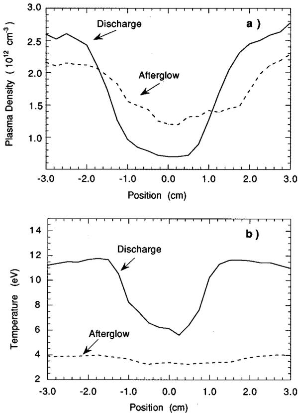
FIG. 2. Radial profiles of plasma density (a) and temperature (b) on a line through the center of the striation during the discharge and 200  $\mu$ s after the discharge.
