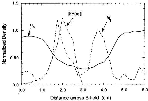
FIG. 8. Radial profiles of fluctuations in the magnetic field-aligned current and the Fourier amplitude (linear scale, arbitrary units) of magnetic field fluctuations superposed on the ion saturation current profile. Only half the magnetic fluctuation profile is shown for reasons given in the text.
