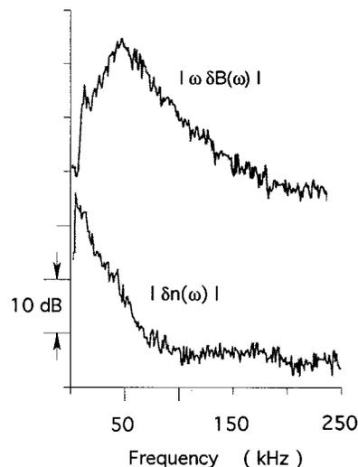
FIG. 15. Frequency spectrum of density fluctuations at the plasma column edge compared to the frequency spectrum of the time derivative of the magnetic field fluctuations (logarithmic scale).
