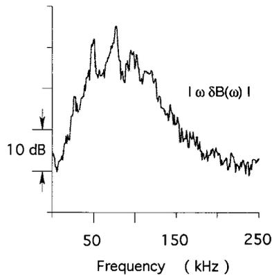
FIG. 16. Frequency spectrum (logarithmic scale) of magnetic fluctuations within the striation at low electron beta (high background magnetic field).
