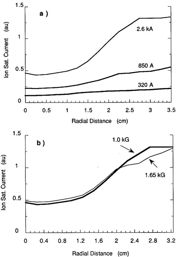
FIG. 4. Changes in the ion saturation current profile of the striation for different discharge currents (a) and different background magnetic field strength (b).
