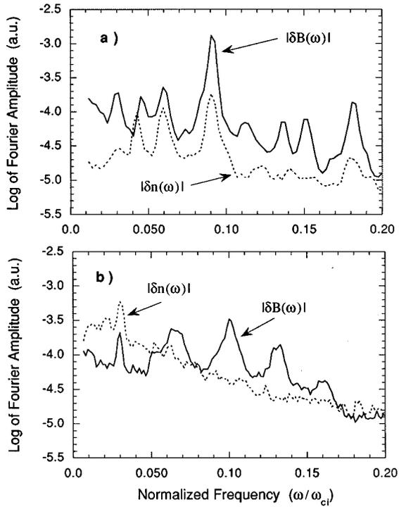
FIG. 12. Frequency spectra of magnetic field fluctuations and density fluctuations for electron beta above the mass ratio (a) and below the mass ratio (b).
