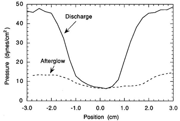
FIG. 3. Pressure profiles in the vicinity of the striation during and after the discharge.
