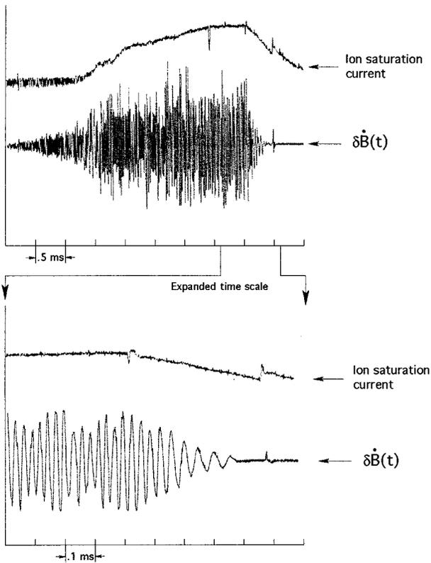
FIG. 6. Temporal development of the magnetic fluctuations and the plasma density. The expanded time scale illustrates the coherency of the magnetic signal and its decay when the discharge is terminated.
