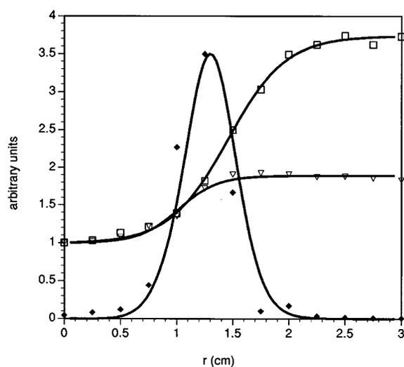
FIG. 17. Theoretical prediction (solid curve) of the radial profile of density fluctuations ( $|\delta n|^2$ ) compared to observed values (solid diamonds). Inverted triangles are measurements of electron temperature and squares are plasma density. Solid curves through these data points represent analytical fits used in the theoretical calculations.
