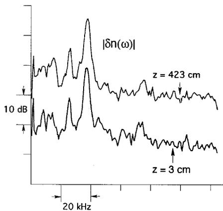
FIG. 9. Frequency spectrum (logarithmic scale) of density fluctuations in the density gradient region of the striation at two axial locations as noted.
