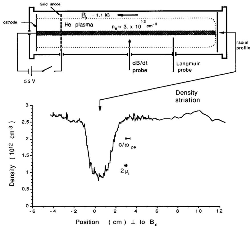
FIG. 1. A schematic representation of the experimental setup. A density striation running the entire length of the machine is created by selective coating or masking of the cathode. A radial density profile in the vicinity of the striation shows the density gradient scale length is on the order of the electron skin depth.
