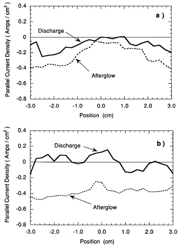
FIG. 5. Radial profiles of the magnetic field-aligned current in the plasma during and after the discharge with a density striation (a) and without a striation (b).
