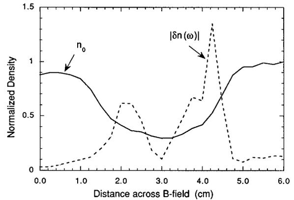
FIG. 7. Radial profile of the Fourier amplitude (linear scale, arbitrary units) of density fluctuations for the frequency corresponding to the peak amplitude ( $\approx 37$  kHz) superposed on the ion saturation current profile.
