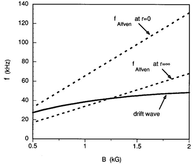
FIG. 13. Theoretical dependence on the strength of the background magnetic field of the frequency of the dominant drift-wave eigenmode (solid curve) and the minimum Alfvén wave frequency inside and outside the striation (dashed curves).
