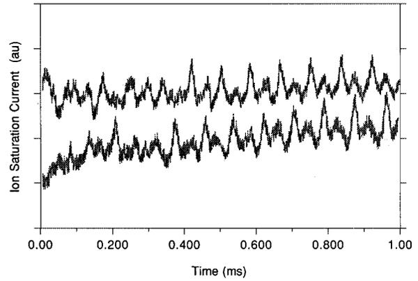
FIG. 10. The temporal behavior of the ion saturation current measured at two diametrically opposed points in the density gradient region of the striation.
