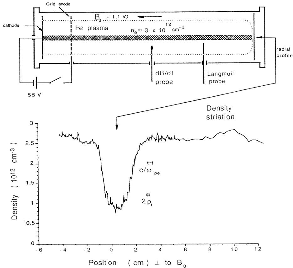
**Figure 1.** Experimental set up. Top: schematic of the plasma device (LAPD). Bottom: expanded view of the radial density profile of a controlled density filament whose axial extent is 10 m (the full length of the device).
