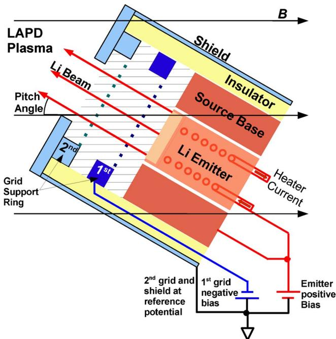
FIG. 1. (Color online) Cross sectional view of a generic lithium ion source in the LAPD plasma at a pitch angle of  $30^\circ$ . Shaded area corresponds to the beam extraction region, which is also the domain used to simulate the field line configuration in Fig. 4.
