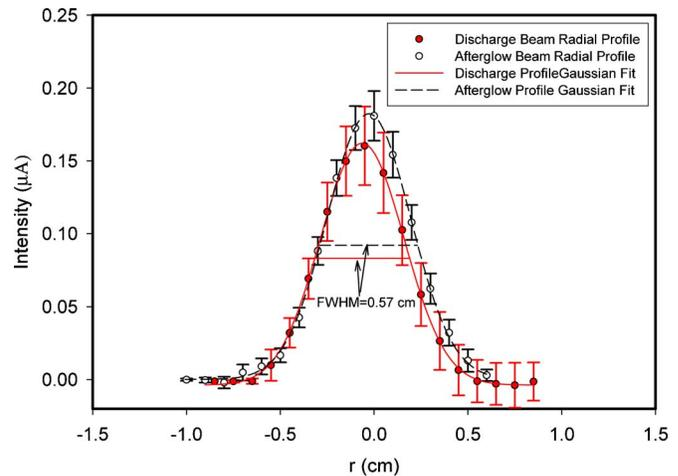
FIG. 10. Weighted average radial beam profile in the discharge and the afterglow.  $r=2.7$  cm corresponds to the predicted center of the gyro orbit. The horizontal line indicates the FWHM for each curve.
