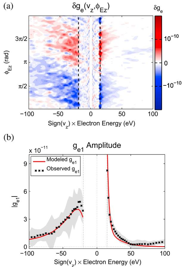
**Figure 4.** The composite measurement of  $g_e(v_z)$  is generated using 64 phase-shifted data sets. (a) Sorting measurements by Alfvén wave phase and electron energy show that there are modifications of the electron distribution  $\delta g_e = g_e - g_{e0}$  at the frequency of the Alfvén wave. (b) Magnitude of the first Fourier mode with respect to Alfvén wave phase compared to the solution of equation (2).
