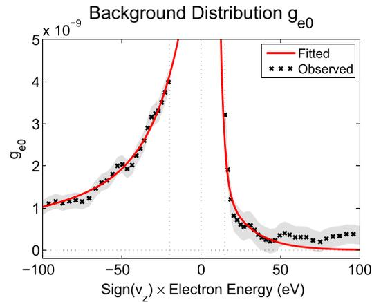
**Figure 3.** The measured background distribution function  $g_{e0}$ . Systematic errors, shown shaded, are due to whistler ducting. Dashed lines near +15 eV and -20 eV are the low-energy limit of WWAD measurements.
