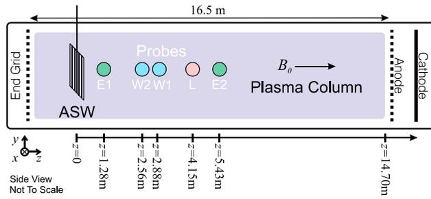
**Figure 1.** Experimental setup in the LaPD. Elsasser probes E1 and E2 observe the perpendicular wavefields  $\mathbf{B}_\perp$  and  $\mathbf{E}_\perp$  in the  $x$ - $y$  plane. Whistler probes W1 and W2 are used to measure the parallel electron distribution function  $g_e(v_z)$ . A scanning Langmuir probe, denoted as  $L$  above, measures electron density and temperature.
