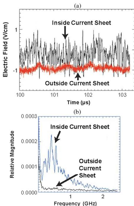
Fig. 5. Electric-field measurements of probes in a plasma current sheet. (a) Electric-field fluctuations over time. (b) Spectral plot of the time sequence shown in (a).
