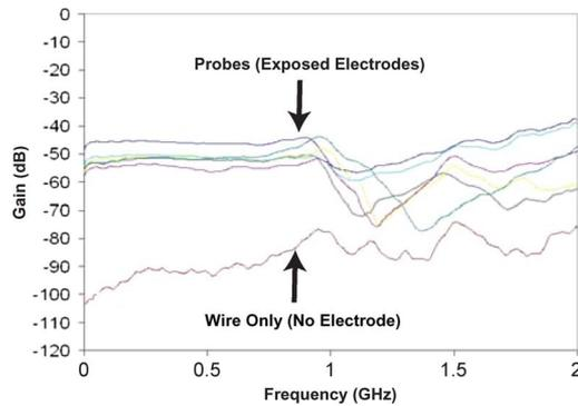
Fig. 4. Frequency response of six individual voltage probes and a probeless wire mounted on a preamplifier circuit board and driving the probe-shaft feedthrough wiring.
