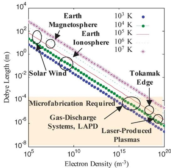
Fig. 1. Debye lengths of some types of plasmas as a function of temperature and density.
