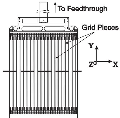
FIG. 1: This is a schematic view of the dispersive Alfvén wave antenna as seen along the  $z$ -axis of the LAPD. Each grid is made of copper mesh, and they are separated by 0.635 cm. Each grid may be driven separately, allowing good control over the perpendicular wave number. The dashed line shows the  $\hat{x}$  and  $\hat{y}$  positions at which raw data is acquired by b-dot probes placed at several  $\hat{z}$  positions.
