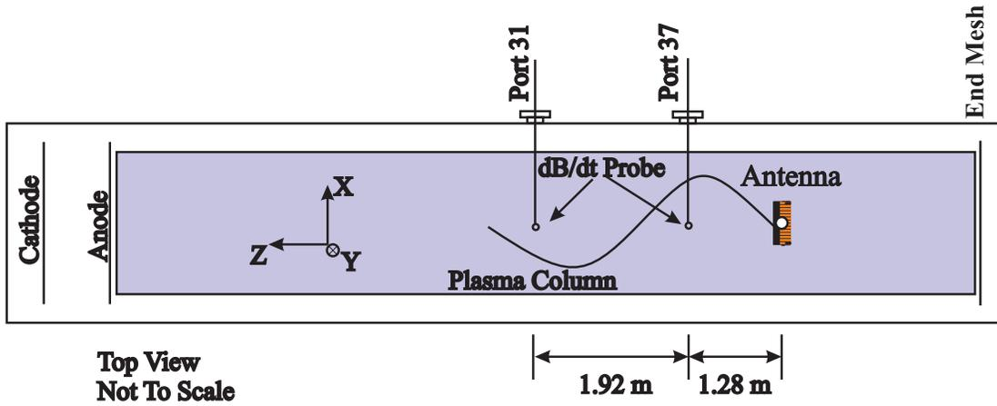
FIG. 3: (Color online) This schematic shows the placement of the b-dot probes with respect to the cathode and antenna. Waves are launched toward the cathode. The wave is then measured by two probes separated by a couple of meters.
