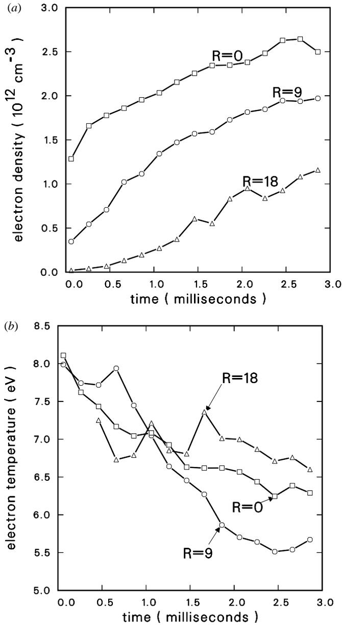
**Figure 2.** Measured values of electron density (a) and temperature (b) as a function of time at radial positions of  $R = 0, 9,$  and  $18$  cm from the centre of the LAPD plasma column.
