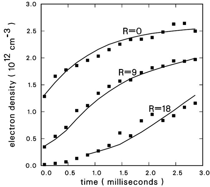
**Figure 3.** Comparison of the calculated electron density (full curve) with measured values (boxes) as a function of time for  $R = 0, 9,$  and  $18$  cm from the centre of the plasma column.
