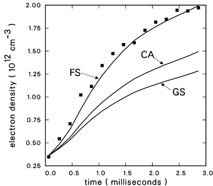
**Figure 4.** Comparison of the measured electron density at  $R = 9$  cm as a function of time with calculations using different atomic models. FS is the fine structure model, CA is the configuration average model, and GS is the ground state model.
