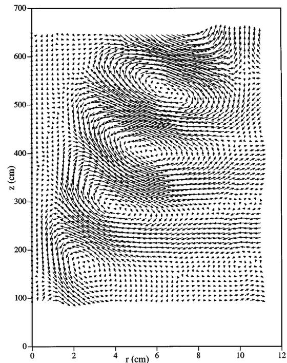
FIG. 3. The product  $r\mathbf{j}(r, z)$  is presented at an instant of time.  $\mathbf{j}$  is calculated for the case with  $\beta_e m_i/m_e = 6.8$ . The source is located at  $z = 0, r = 0$ , and has a  $0.5$  cm radius. The centers of the vortices are located  $1.25$  m or  $\lambda_{||}/2$  apart.
