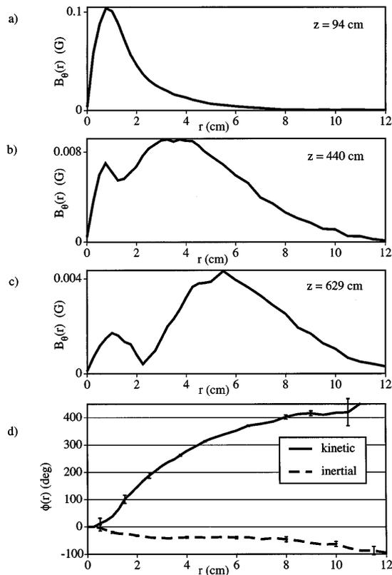
FIG. 2. (a), (b), and (c):  $|B_\theta(r)|$  for the case with  $\beta_e m_i/m_e = 6.8$  at several  $z$  positions.  $|B_\theta(r)|$  is the amplitude of the azimuthal component of the wave magnetic field. (d) Phase of  $B_\theta$  as a function of  $r$ ,  $\phi(r)$ . The solid line is for the case with  $\beta_e m_i/m_e = 6.8$  (at  $z = 440$  cm), and the dashed line is for the case with  $\beta_e m_i/m_e = 0.23$  (at  $z = 189$  cm; amplitude profile not shown).
