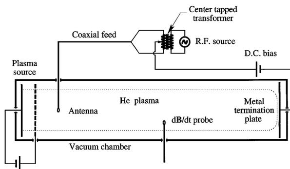
FIG. 1. During the experiment, the termination plate is at plasma floating potential; the dc bias holds the disks up near the plasma potential while the rf source drives the oscillating current.
